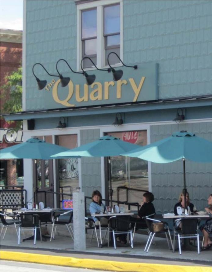
Above, signage lighting is shielded and directed onto the building and sign.
