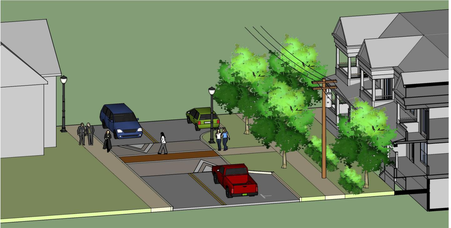
Axonometric View of Sidewalk 'Bump-Out' and raised crosswalk.
